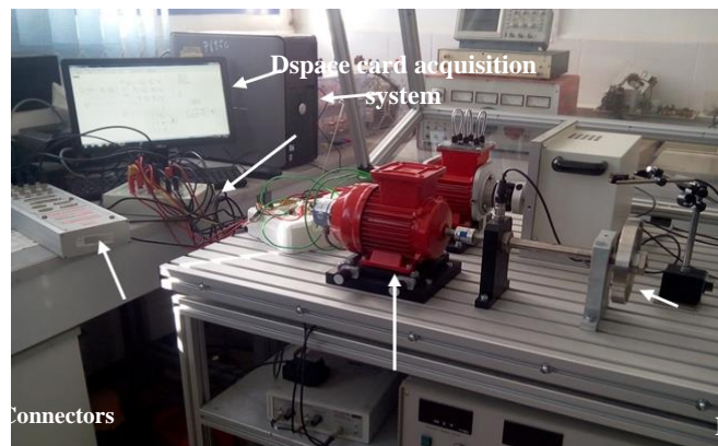
Figure 2. Experimental setup (composed of a 0.37 kW induction machine supplied by an inverter)
