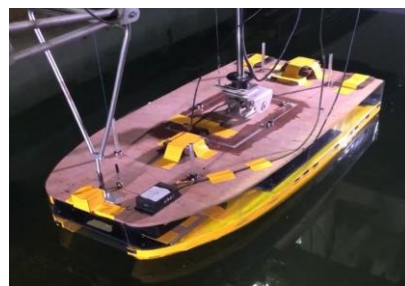
Figure 3. USV Catamaran model setup for resistance test
