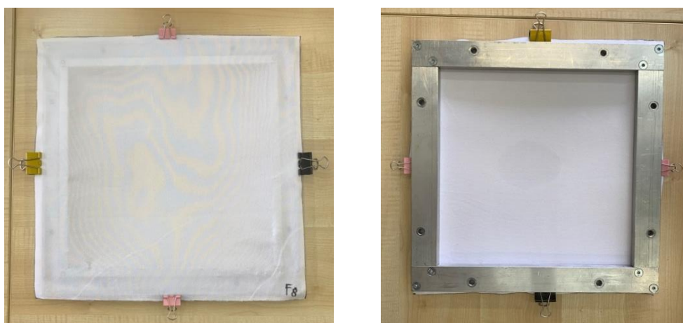
Figure 1. Setting up the fabric for the tests with the frame
